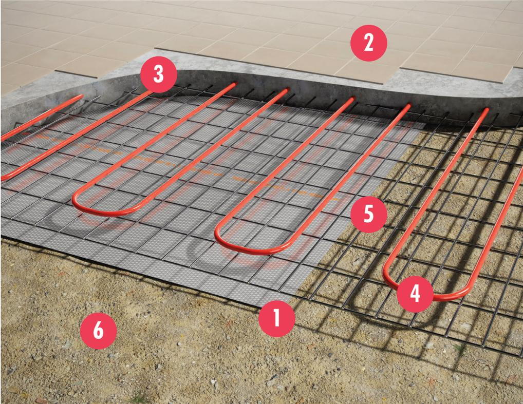
1. Reflectix® Concrete Slab Insulation
