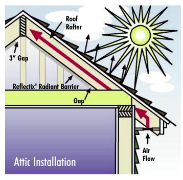
Staple product to the bottom of the rafters, overlap seams 2" and insure a gap at the peak (3") and along lower roof line (as convenient depending on roof pitch). Additionally, install product across gable studs. An alternative installation (Southern USA only) would involve stapling the product directly to the decking between the rafters (or trusses) as depicted in the Alternate Attic Installation (upper right).
