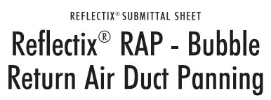
Reflectix® RAP (Bubble) is an alternative to conventional sheet metal and corrugated aluminum panels for return air ducts. In wood frame construction, it may be used to enclose the bottom of return air plenums, between the joist spaces, stud cavities, and wall and ceiling cavities.
