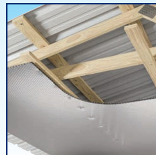
Roof / New / Retro* (Bottom of Trusses) R-10 Heat Flow Down R-3.7 Heat Flow Up
