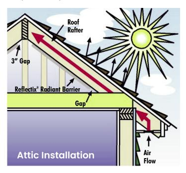
Staple product to the bottom of the rafters, overlap seams 2" and insure a gap at the peak (3") and along lower roof line (as convenient depending on roof pitch). Additionally, install product across gable studs. An alternative installation (Southern USA only) would involve stapling the product directly to the decking between the rafters (or trusses) as depicted in the Alternate Attic Installation (upper right).
