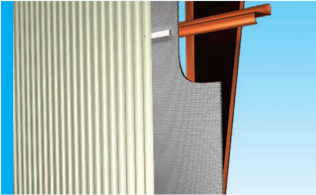
Wall / New (Thermal Break) R-6.0
