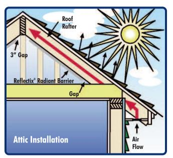
Staple product to the bottom of the rafters, overlap seams 2" and insure a gap at the peak (3") and along lower roof line (as convenient depending on roof pitch). Additionally, install product across gable studs. An alternative installation (Southern USA only) would involve stapling the product directly to the decking between the rafters (or trusses) as depicted in the Alternate Attic Installation (upper right).
