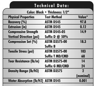
Meets Application Requirements of: ASTM D 1752 Sections 5.1-5.4 (with the compression requirement modified to 10 psi minimum and 25 psi maximum.) ASTM D 4819 Type II
