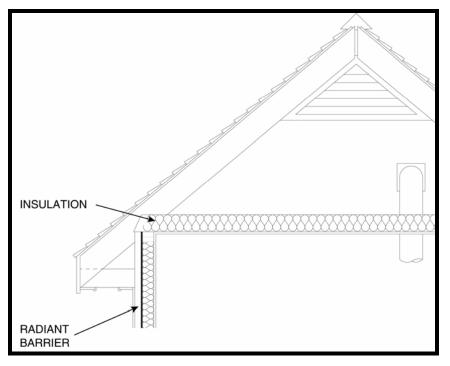
**TECHNICAL NOTE**: Radiant barriers which are non-perforated are vapor barriers. Care should be exercised with placement!
