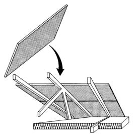
3. Horizontal installation (directly above ceiling and/or ceiling insulation)
