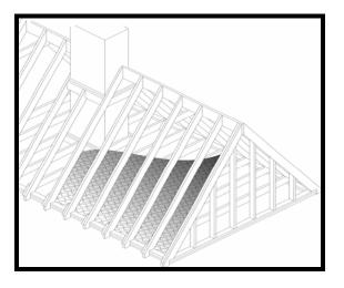
A Typical Attic Installation for Reflective Insulation
