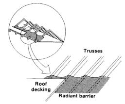
A radiant barrier can be draped over the trusses with the foil facing down.
